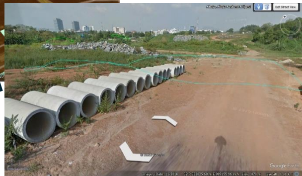
Figure 7. Street View ground-truth confirmation: the objects circled in overhead imagery are stacked concrete culvert/pipe segments, not buildings
